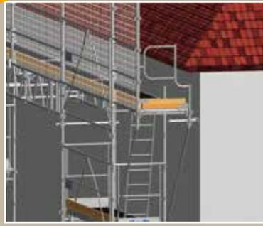
**UN ÉCHAFAUDAGE ADAPTÉ AUX TRAVAUX DE COUVERTURE AVEC UNE PROTECTION RENFORCÉE EN BAS DE PENTE DE TOIT.**
